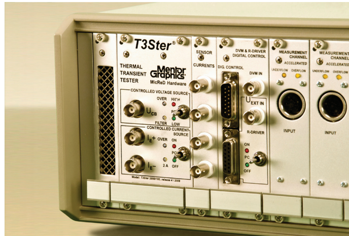
Figure 9: Mentor Graphics T3Ster Thermal Transient Tester captures the transient response of an LED after just 1 \mu\text{s} ( 1 \times 10^{-6} seconds), with a temperature resolution of 0.01 ^{\circ}\text{C} .
