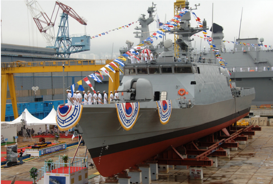
Caption: Gumdoksuri class offshore patrol vessel Yoon Youngha (PKG 711) being launched.
