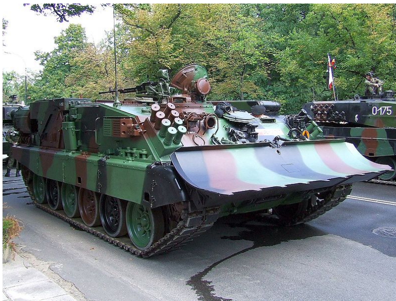
The WZT-3, built on a T-72M hull, will provide the manufacture basis for India's new recovery vehicles
