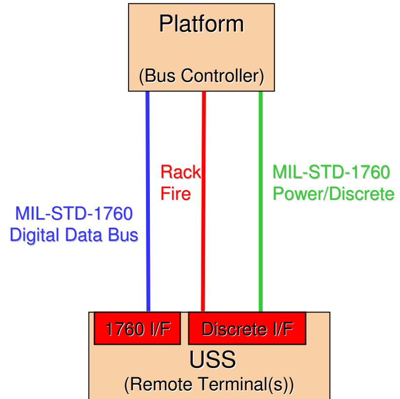
*The USS is an extremely versatile test tool designed to fully validate a UAI Platform interface*
