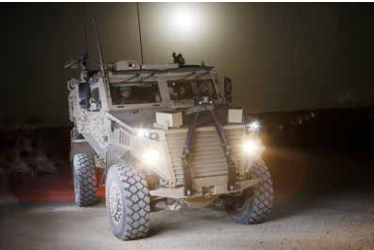
The UK's Foxhound is engineered using a variety of composites, both structure and armour Source: Ministry of Defence
