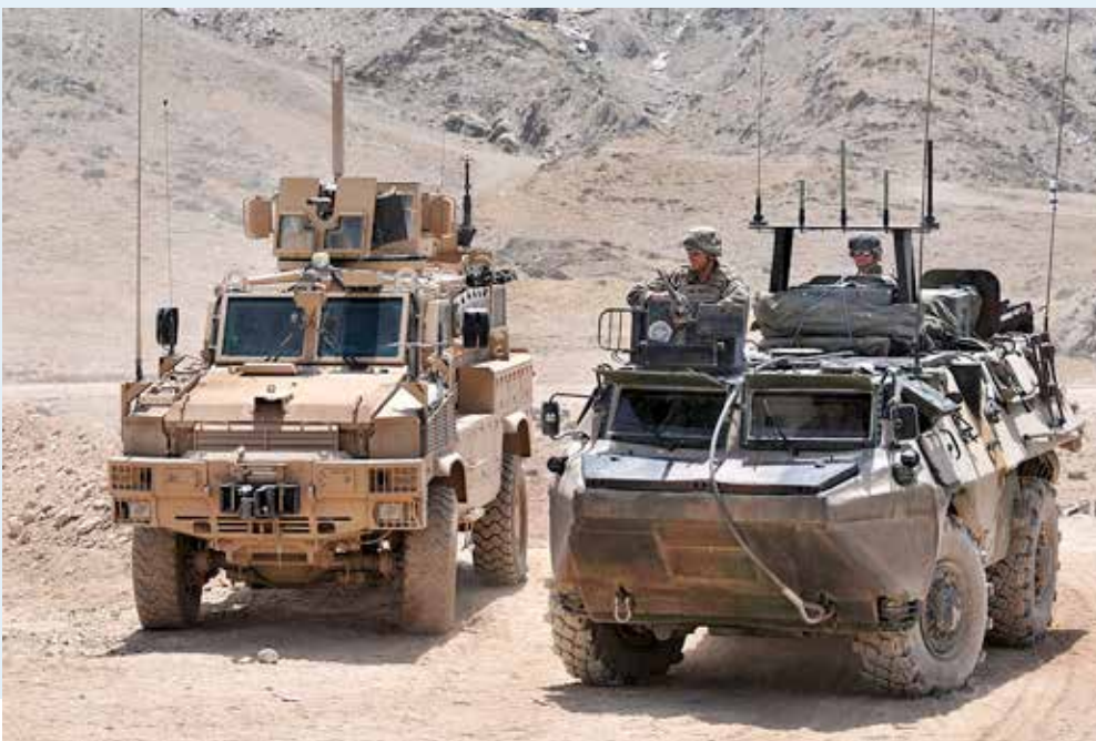
An outgoing French VAB, shown on the ISAF mission alongside a US Army MRAP, soon to be replaced by the VBMR
