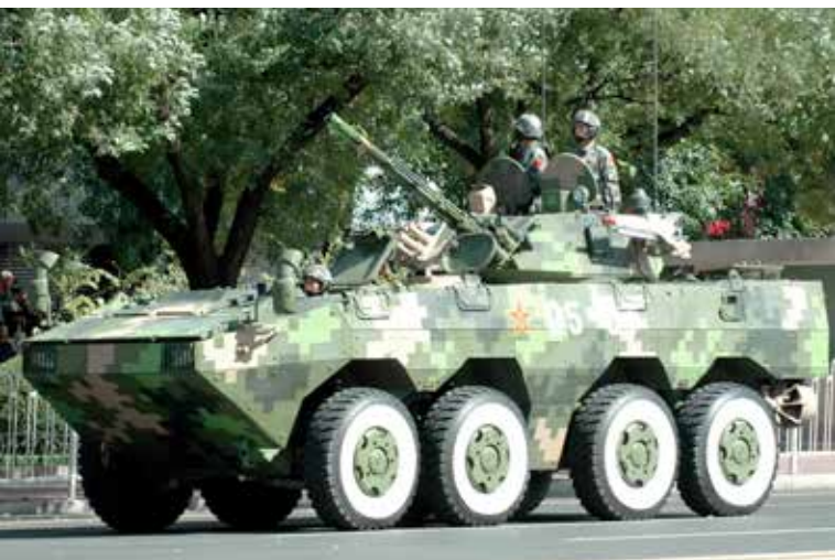
The Venezuelan VN-1 8x8 APC is the export version of the Chinese ZBL-09
