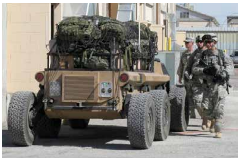
U.S. soldiers test the (now cancelled) Multifunctional Utility/Logistics and Equipment (MULE) UGV, designed to support dismantled, mounted and air assault operations. R&D has since been spent on Google's 'Big Dog' legged robot mule. Source: U.S. Army
