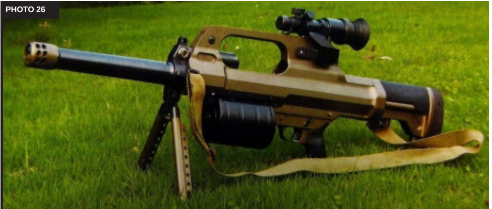
LG3 belt-fed automatic grenade launcher chambered for the 40 x 53 mm cartridge. Photo Credit: SINA Corporation
