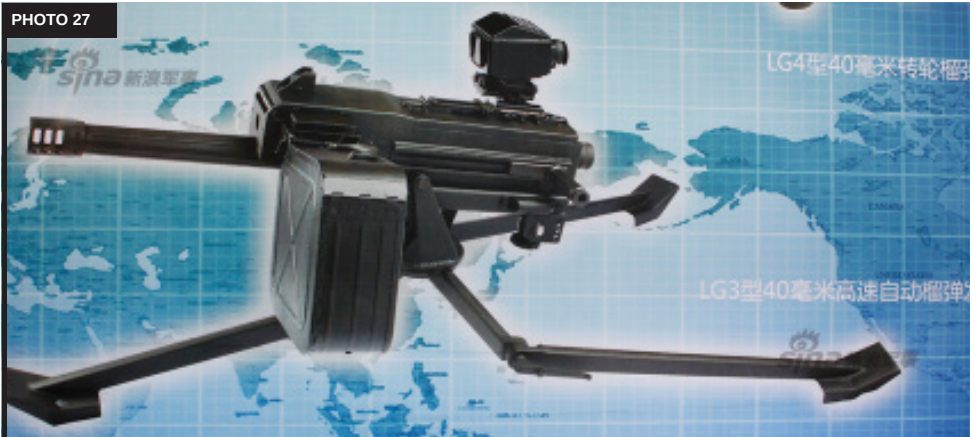
LG3 belt-fed automatic grenade launcher chambered for the 40 x 53 mm cartridge. Photo Credit: SINA Corporation
